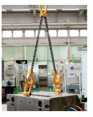
Seating face contact is essential for the eye bolt, but the ring direction is inconsistent...
